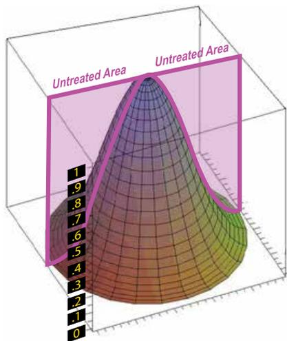
The picture above shows the typical electromagnetic field for one of the flat coils placed inside a therapy mattress. As you move away from the coil the magnetic field diminishes. This means that although the pulsing field will completely penetrate the body, some “dead” areas will occur (as shown in the purple areas of the picture).
