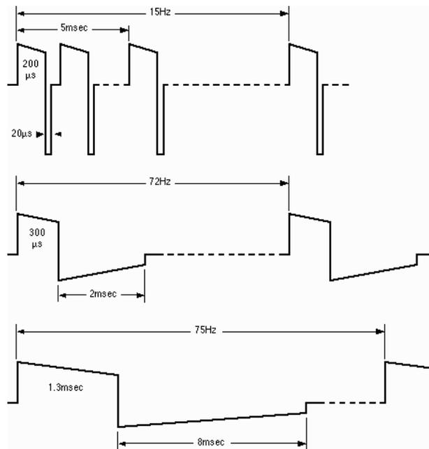
**Figure 2:** Induced electric field,  $E(t)$ , in tissue from the time-varying magnetic fields utilized in EMF devices for clinical applications. The top waveform consists of bursts of asymmetrical pulses; the others are wide asymmetrical single pulses. For all signals peak  $E$  is 1-10 mV/cm in a 2 cm target. All are detectable by some tissue targets. Positive clinical effects have been reported for all signals.
