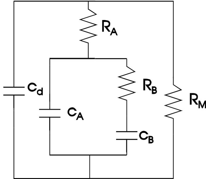
**Figure 4:** Electrical equivalent circuit of a cell membrane which exhibits a dielectric membrane capacitance,  $C_d$ , a leak resistance,  $R_M$ , an ion binding pathway having an equivalent resistance,  $R_A$ , and capacitance,  $C_A$ , and a time constant,  $R_B C_B$ , representing a coupled surface step, e.g., conformation change. This circuit requires ion binding to occur prior to the follow up step.
