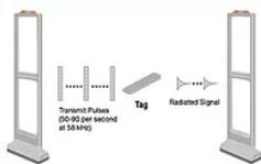
In Acousto-magnetic systems the transmitter sends a RF signal of ~ 58 kHz in pulses to energize the tag in the surveillance zone.
