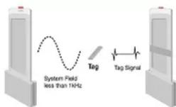
In Electromagnetic (EM) systems a magnetic strip is attached to the goods.
