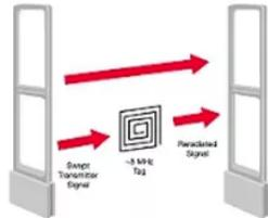
In Radio Frequency (RF) Systems a label (miniature disposable electronic circuit and antenna) attached to a product responds to a specific frequency emitted by a transmitter.
